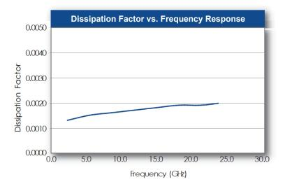
robustness of Rogers' laminates across frequency, thus simplifying the final design process when working across EM spectrum. The stability of the dielectric constant of TC350 laminate over frequency ensures easy design transition and scalability of design.
