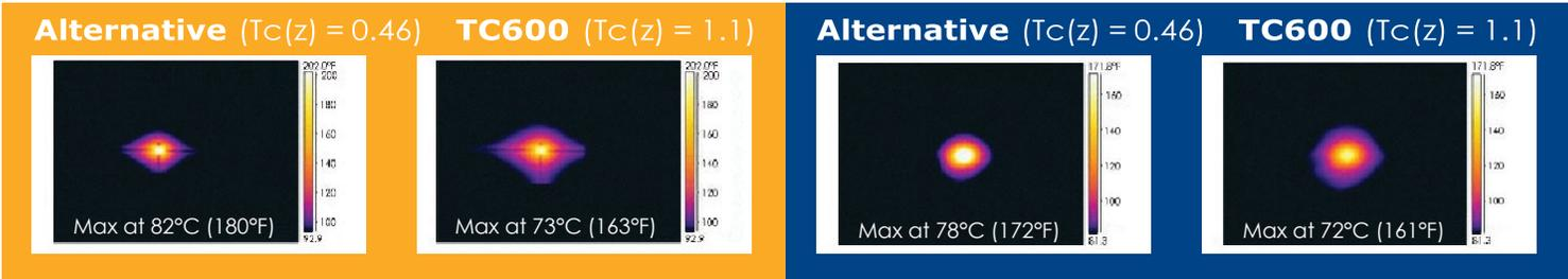
Figure 3 - THERMAL COMPARISON – thermal image of 25 mil laminate test circuit
